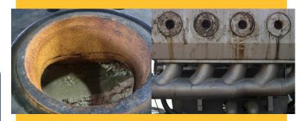
**Left**: Inside suction manifold is a failing weld, and is packed with sand. **Right**: A failed FE with attached 5-port suction manifold.
